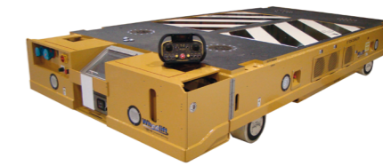
A 140-ton, eight-module headless transporter with Autec's remote control
