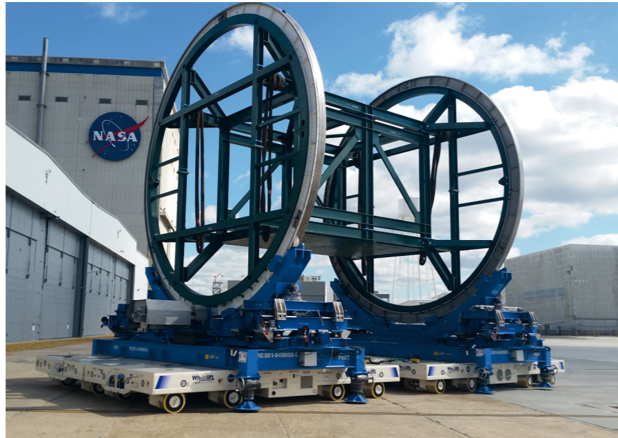
Wheelift transporters are used by NASA for moving space hardware
