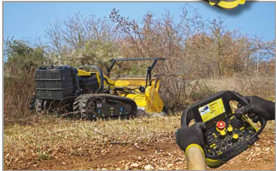
ABOVE: Customized radio remote control with 4.3in color display
